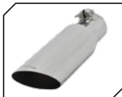
3.50"/2.50"/13.00"L Turn Down - Round Single Wall - Clamp-On Part# 15374 (ea.)
