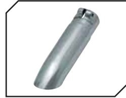
2.75"/2.50"/10.00"L Turn Down - Round Single Wall - Clamp-On Part# 15379 (ea.)
